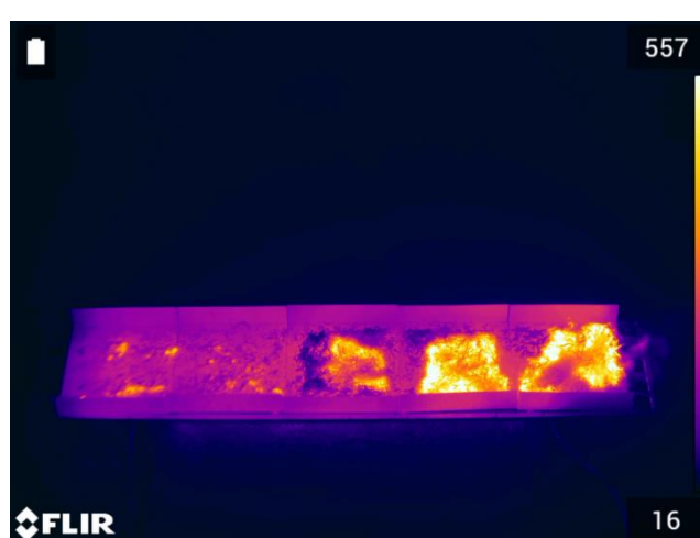
Figure 6. Test 8 – Pine needles, with NoIgnis in Powder to Mix at 557°C
