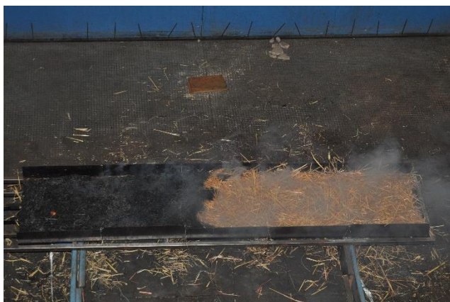
Figure 8. Test 5 – Straw, photo taken after flame extinction at the beginning of the treated bed
