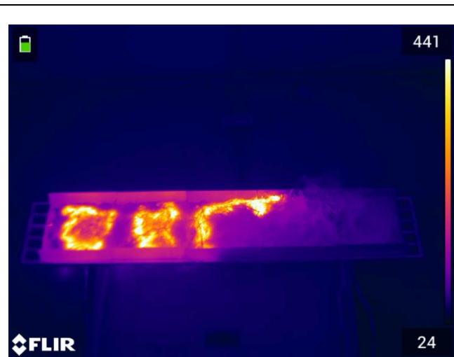
Figure 3. Teste 1 - Straw, with NoIgnis, at 441°C
