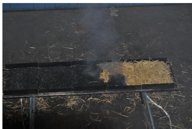
Figure 11. Test 6 - Straw, time at which flames reached the middle of the treated bed with NoIgnis
