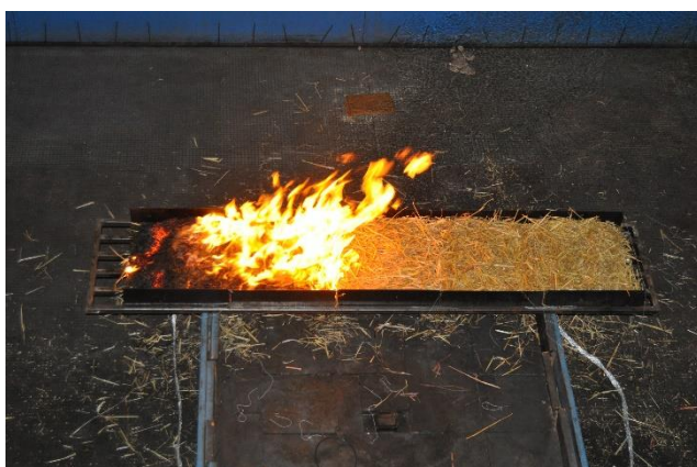
Figure 10. Test 6 – Straw, time at which flames reached the interface between the starter bed and the treated bed with NoIgnis
