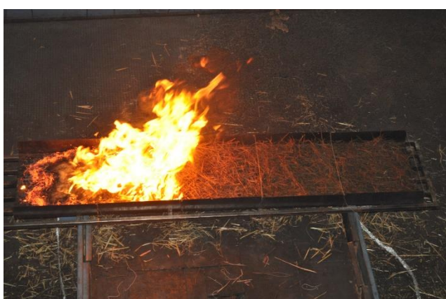
Figure 12. Test 10 – Pine Needles, flame with high intensity and height at the end of the starter bed
