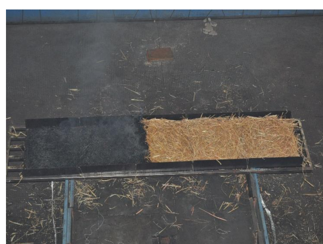
Figure 7. Test 2 – Straw, photo taken after flame extinction at the beginning of the treated bed
