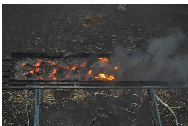
Figure 13. Test 10 – Pine Needles, photo taken at the moment which flames are in the treated bed with reduced size of flames
